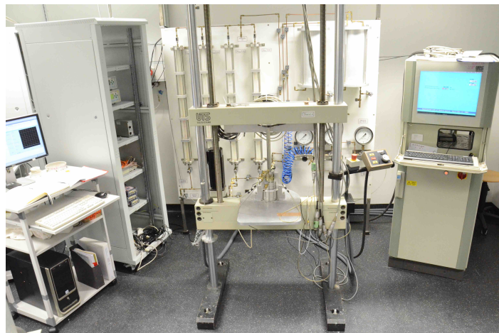
Figure 5.2: UTS control stand: photograph with loading frame (centre), central processing unit (right side) and data acquisition (left side).
