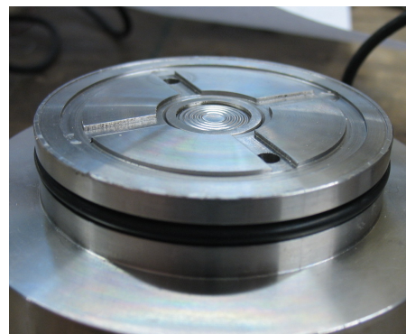
Figure 5.8: Implemented ppt in oedometer bottom.
