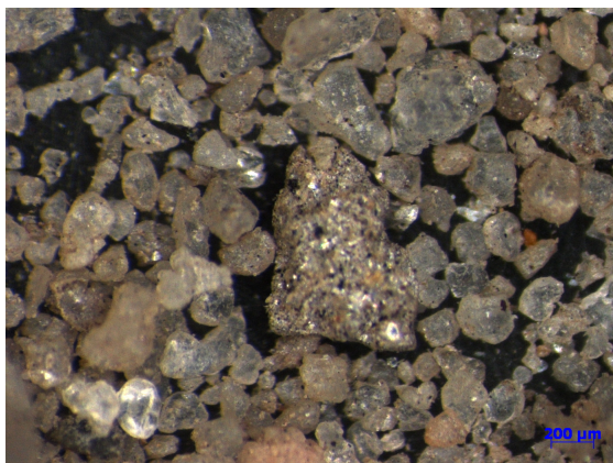
Figure 3.10.: Microscopic pictures of Seese sand (a) 15-049-Schlabendorf-Süd ; (b) 15-050-Seese-West
