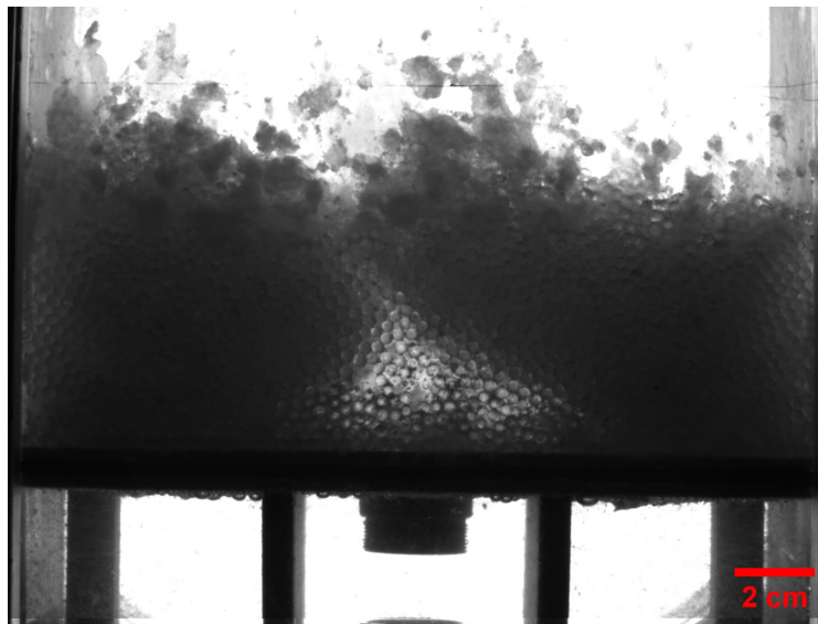
Figure 2.27. – Typical back-light visualization of a cemented granular sample using a led panel.
