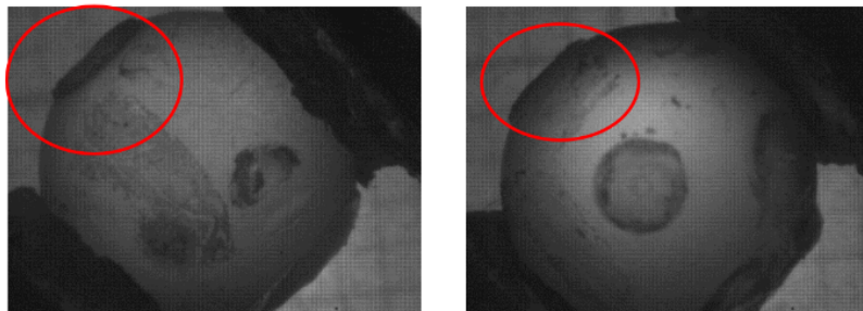
Figure 3.28. – Microscope images illustrating the three different types of rupture after the micro-tensile tests with beads of 7 mm diameter and a paraffin content of X_p = 0.5 %.
