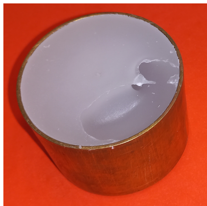
Figure 2.2. – Paraffin volume reduction from liquid to solid.
