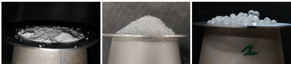
Figure 3.30. – Different shapes of the surface rupture obtained with the large macroscopic cone: (left) almost planar rupture for a sample of 0.6 mm beads with X_p = 0.5\% ; (middle) parabolic shape for a sample of 1.4 mm beads with X_p = 0.2\% ; (right) moderately parabolic shape for a sample of 7 mm beads with X_p = 0.5\% .
