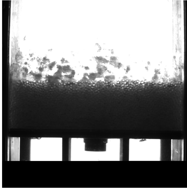
Figure 4.1. – Example of a static regime for a sample with d = 3 mm, Q = 2 l/min and X_p = 0.2 %. Note that the dark spots on the window are paraffin coatings as will be explained later.
