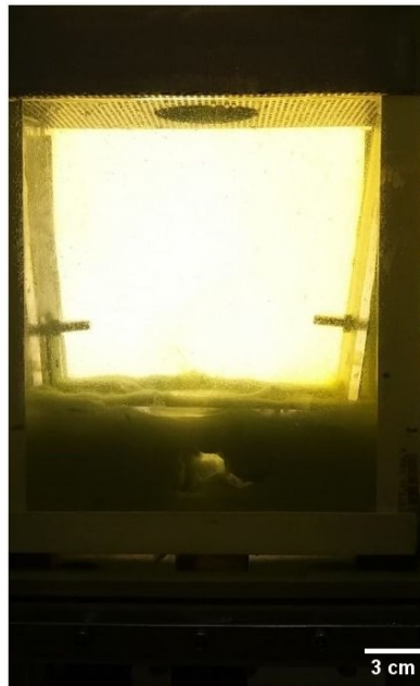
Figure 2.26. – Hydraulic failure within a sample with d=0.1 mm glass beads and X_p = 0.2 % mass paraffin content.
