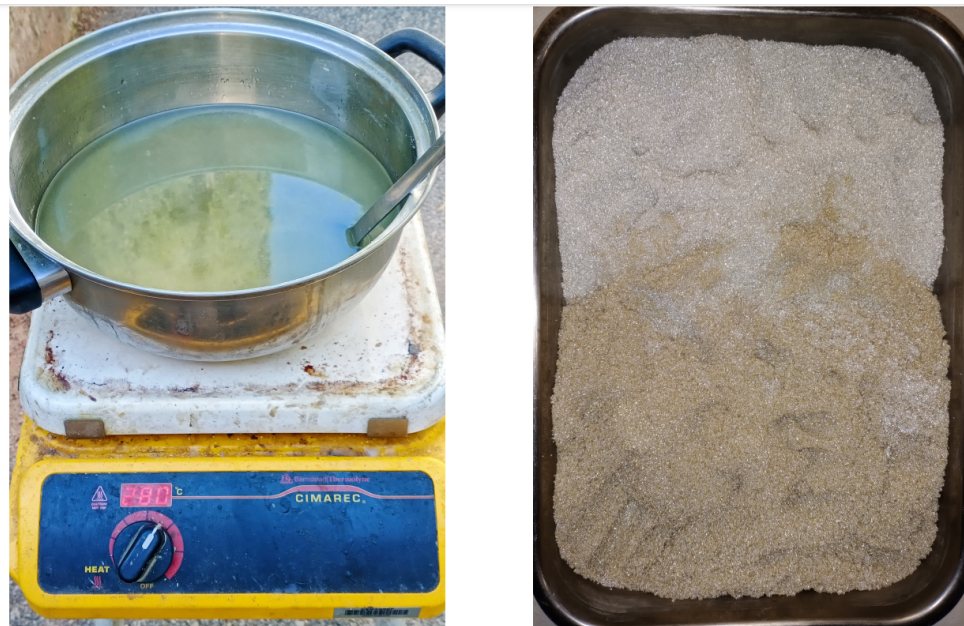
Figure 2.4. – Recycling process: (left) beads immersed in sunflower oil; (right) recycled glass beads.
