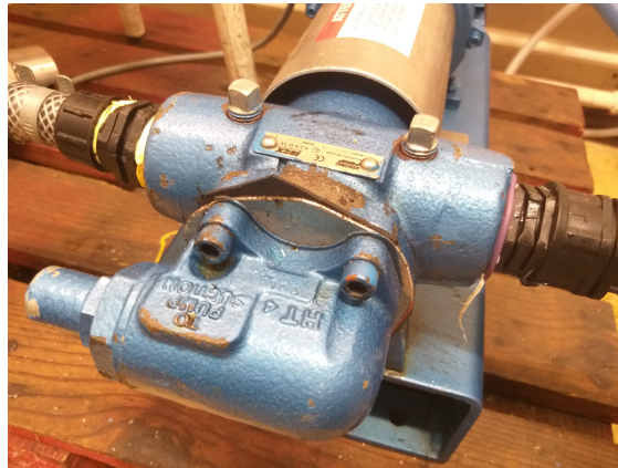
Figure 2.20. – Installation of a latex membrane to exclude the safety block of the gear pump.
