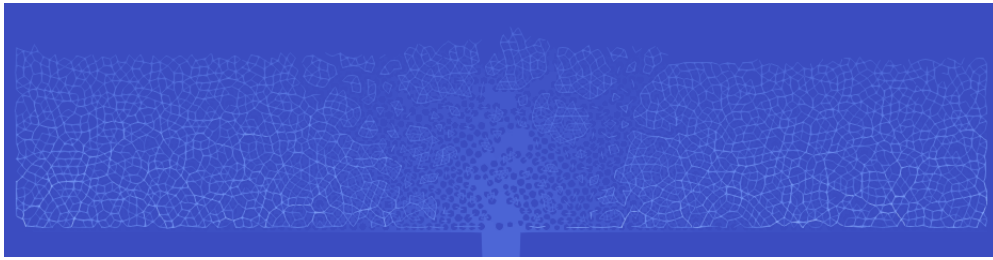
Figure 4.21. – Example of a mixed destabilization scenario for a sample with d = 2 mm, H = 5 cm and \sigma_b = 250 N/m, subjected to an inlet flow rate Q = 1.92 cm 2 /s during 10 s.
