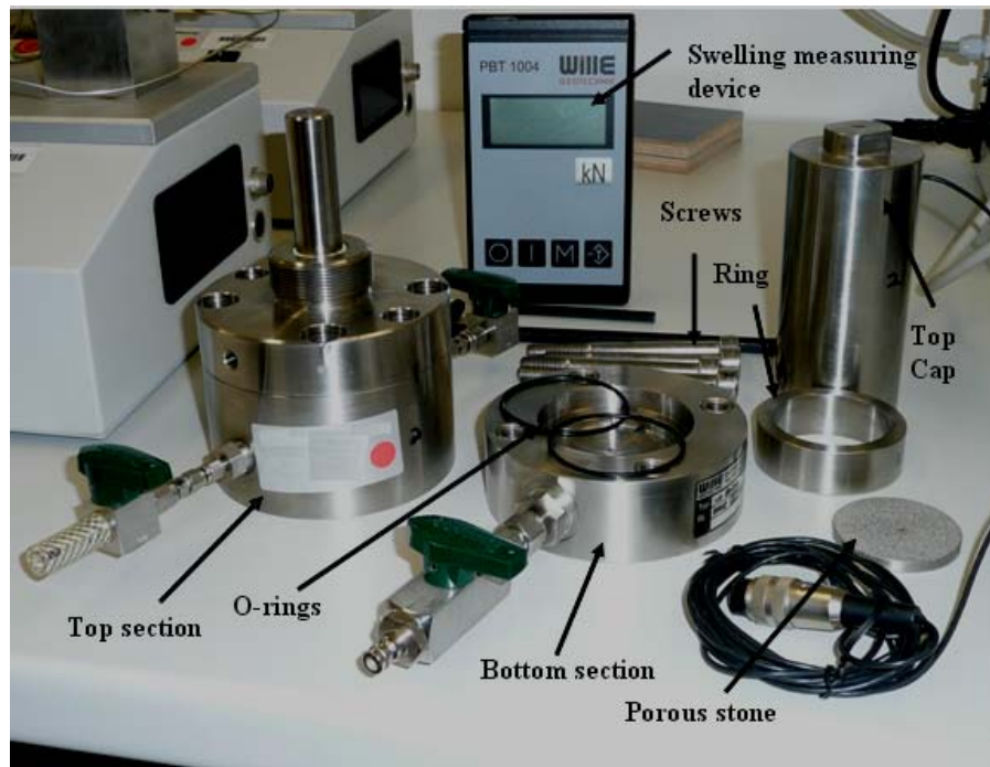
Figure 5.4 Individual components of constant volume device
