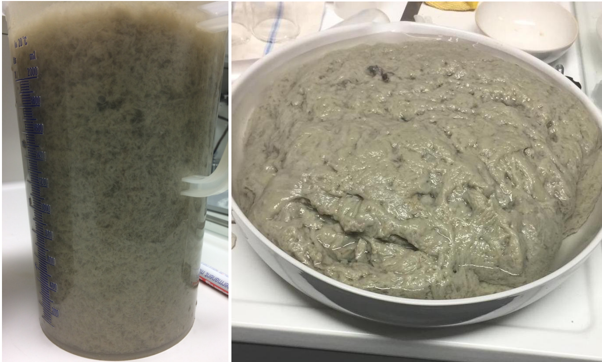
Figure 4.4: Mixtures of the (l.) cationically modified bentonite, and (r.) non-ionically modified bentonite before centrifugation
