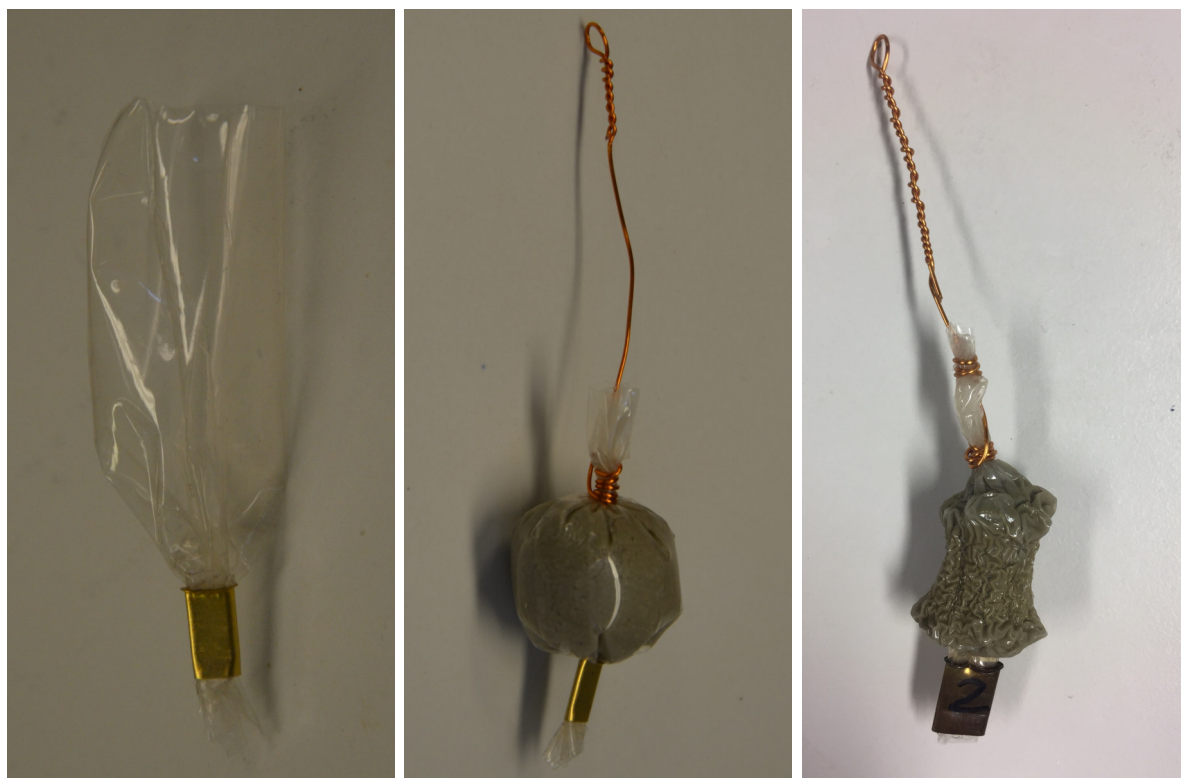
Figure 4.6: Samples for osmotic method (a) empty membrane with brass sleeve, (b) sample at initial conditions inside the membrane, (c) sample after test with visible volumetric shrinkage induced by dewatering
