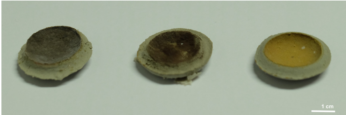
Figure 5.10: \text{PAA}_{S,\tau40}^+ (left), \text{PAA}_{M,\tau40}^+ (middle) and \text{PAA}_{L,\tau40}^+ (right) samples after desaturation at a suction of 328 MPa
