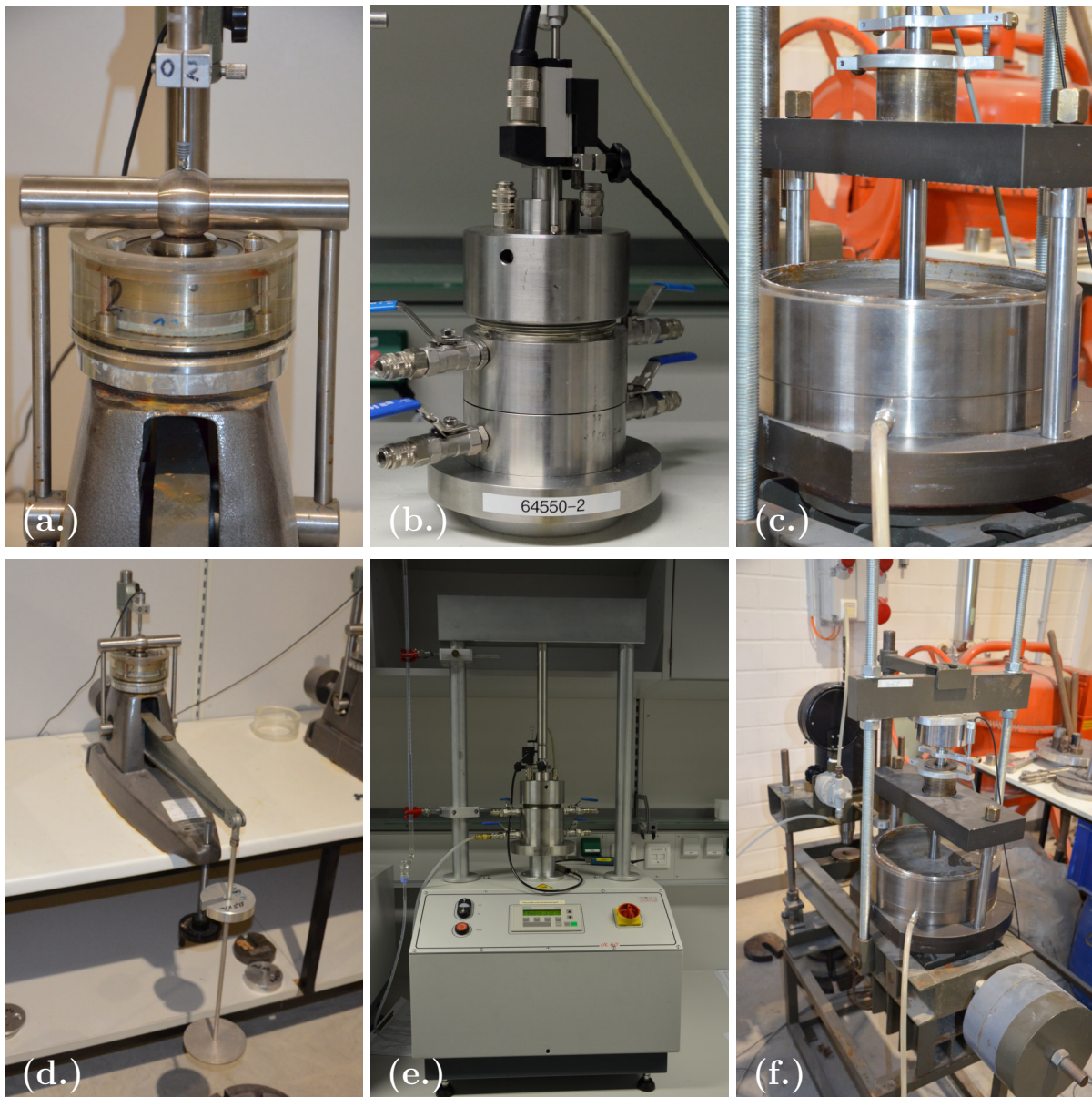
Figure 4.5: The oedometer devices used in the current study (a.), (d.) standard oedometer, (b.), (e.) high pressure oedometer, (c.), (f.) large oedometer. Figures (d.), (e.), (f.) are total views of the devices including the loading frame, and (a.), (b.), (c.) are close-up views of the oedometer cells alone.
