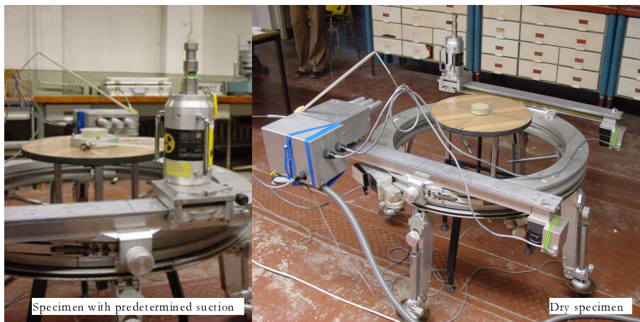
Figure 5.3: Experimental set up for the Computer Tomography (CT)
