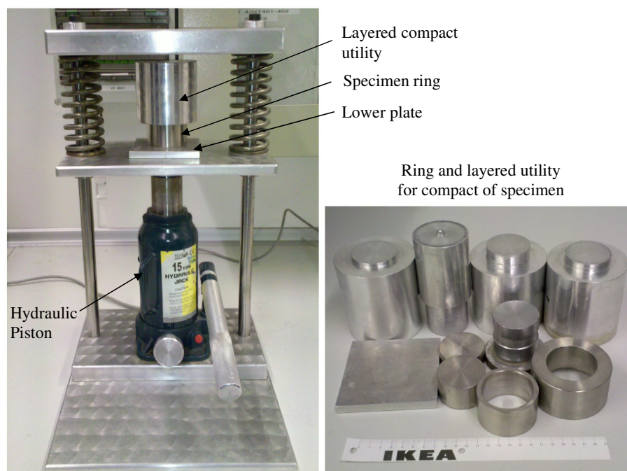
Figure 4.2: Compact device using hydraulic pressure
