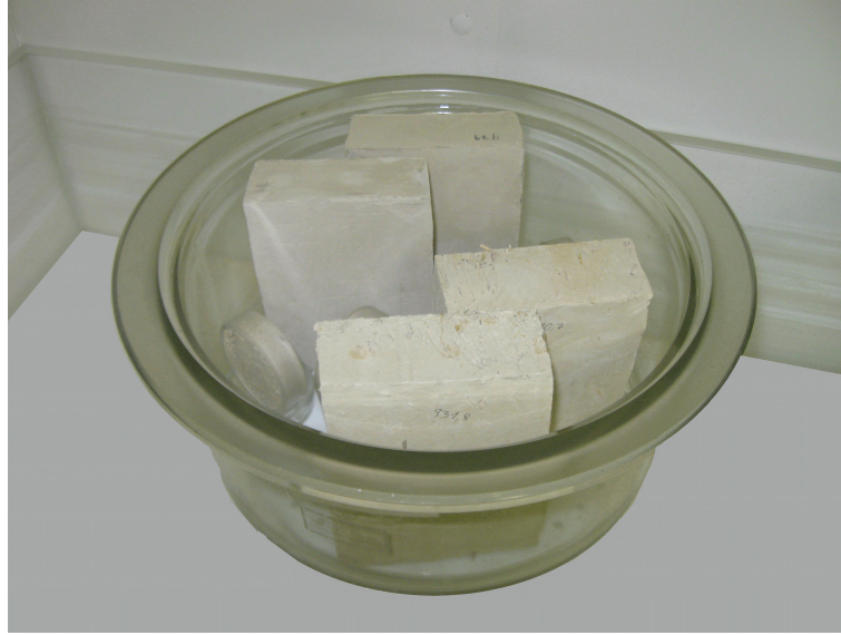
Figure 5.21: Applying suction to the samples with VET method.
