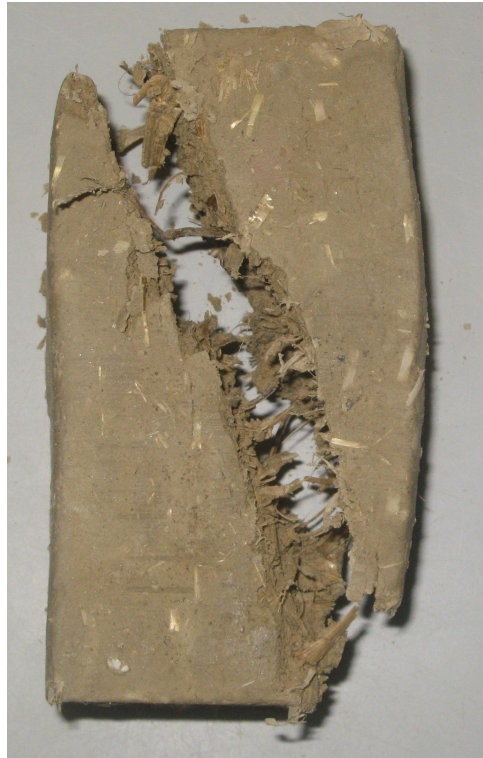
Figure 7.15: Roughness of failure plane caused by straw filaments.
