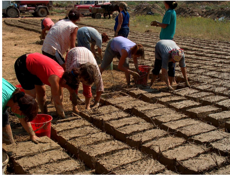
Figure 3.25: Straw inclusion in preparation of adobes.
