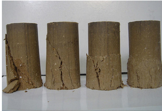
Figure 3.27: Variation of the failure characteristics with fiber content, the fiber content from left to right respectively: 0, 0.05, 0.15, and 0.25 gravimetric percent (Cai et al. 2006).
