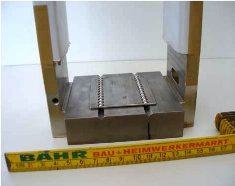
Figure 5.10: Ball bearings and immovable side walls covered with teflon sheets.
